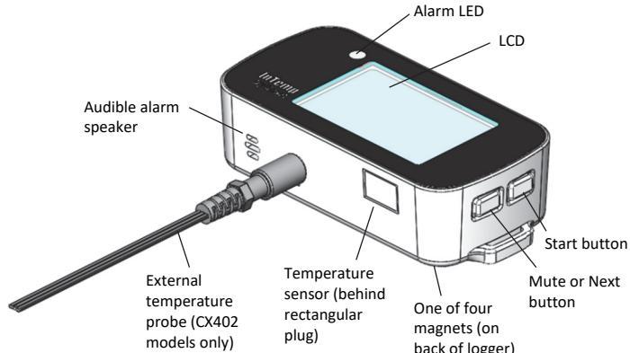
**Start Button:** Press this button for 1 second to start the logger when it is configured to start “on button push.”
