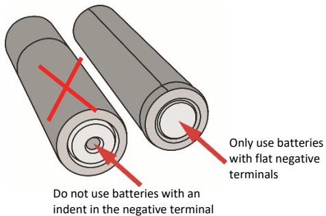
To install or replace the batteries:
