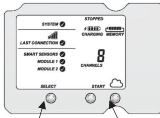
Press the Select button to return to the main LCD screen
