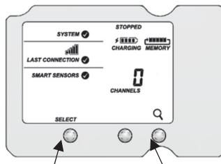
Press the Select button to view the smart sensor channels (pointed out above)
